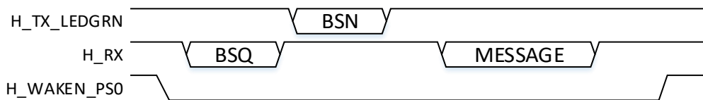
Figure 10: UART-SHTP Sending a message to the FSP200
